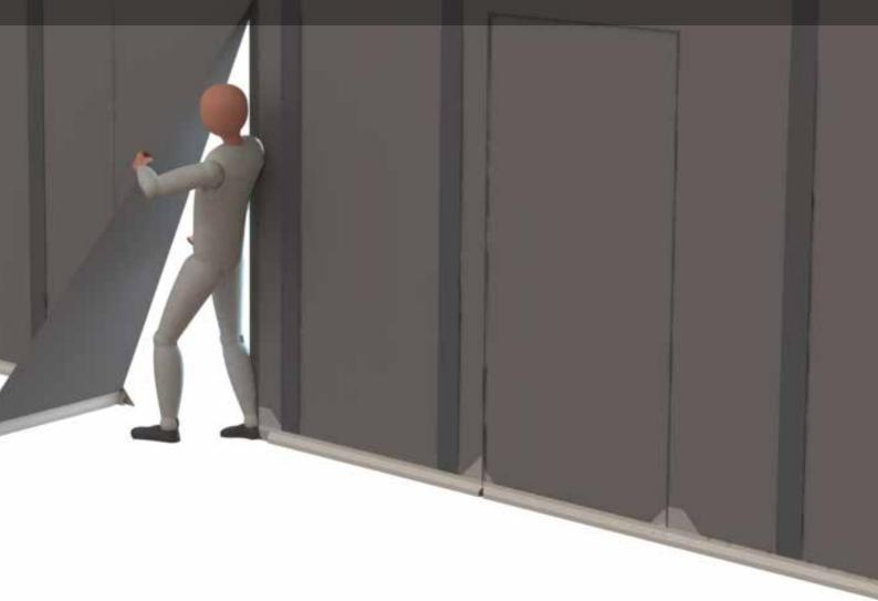
DEPLOYABLE SMOKESTOP EGRESS TESTED TO UL 1784 STANDARD
