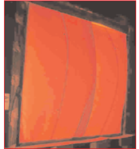
EFP 4/1000 fabric curtain height of 8mtr.
